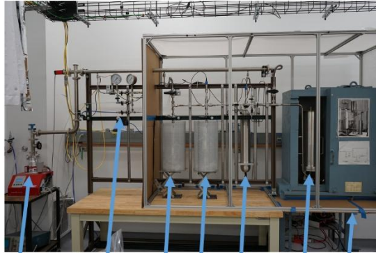
Vacuum Pump Fill Manifold Glass Flask 2 Glass Flask 1 Mixing Volume Counting Cannister Thermal Enclosure
