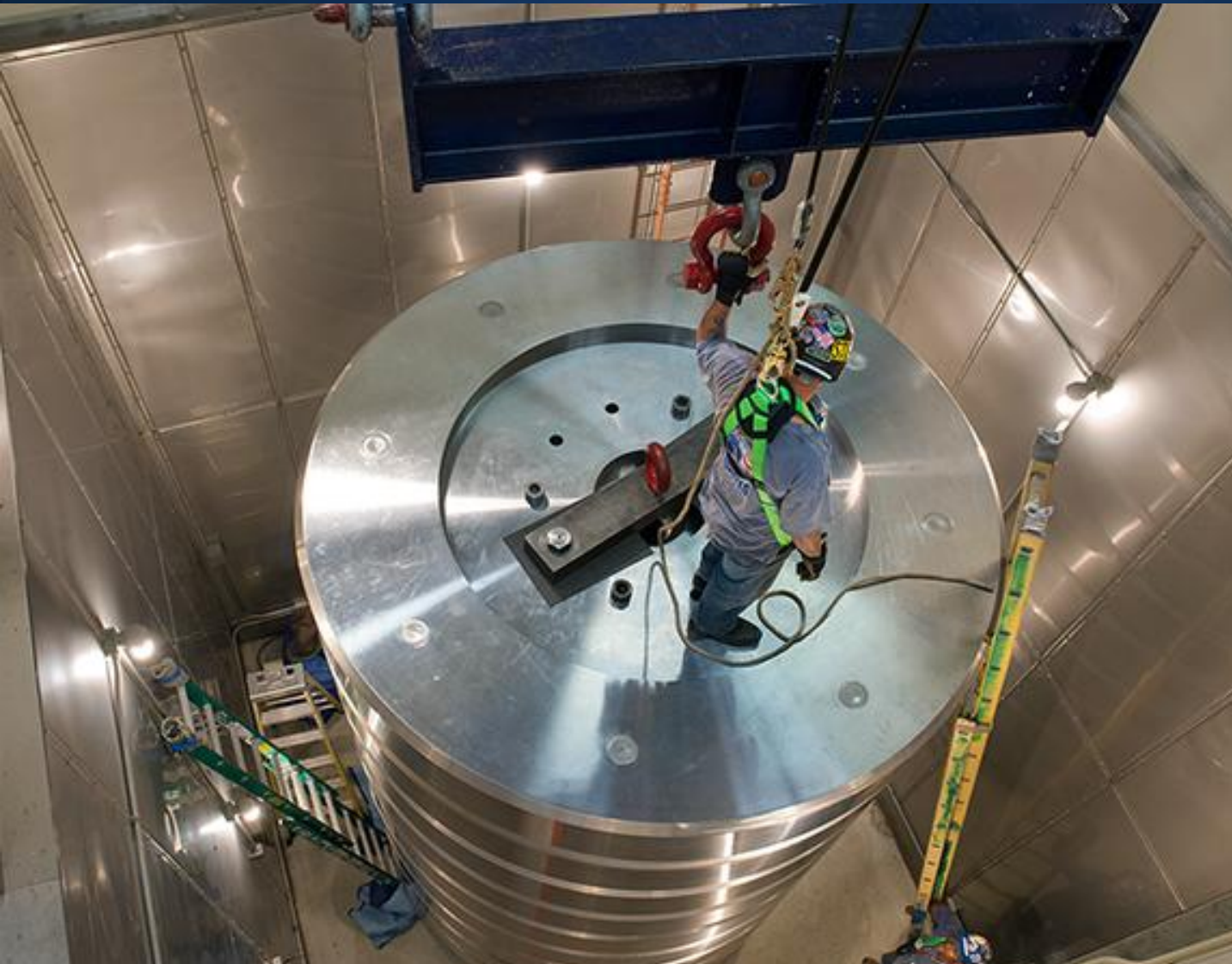
454 ton (Million-Pound) Deadweight Machine
