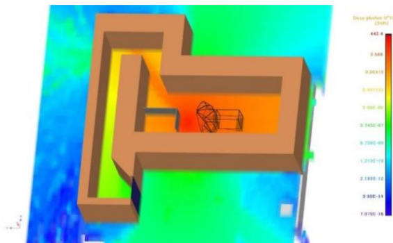
3D mapping of the dose rate around and inside a Co60 bunker
