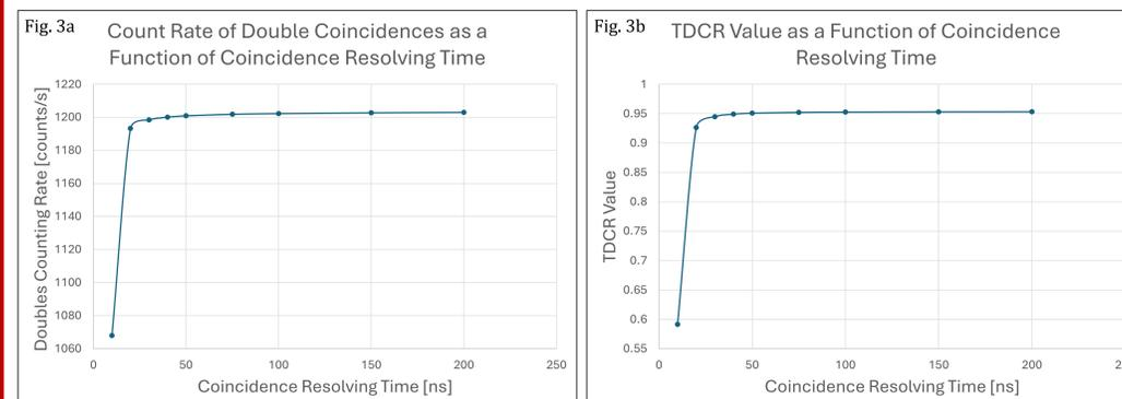
Figure 3: Effect of CRT on double coincidence counting rates (a) and TDCR values (b) done using list-mode data taken with  $^{60}\text{Co}$  source 2 and Filter 0. Post-measurement data analysis available with list-mode data to change CRT and compare observed values.
