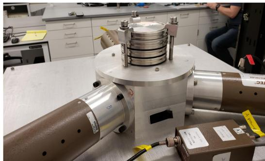
Figure 1. Photo of the TDCR LSC system used by the Radioactivity Group at NIST.
