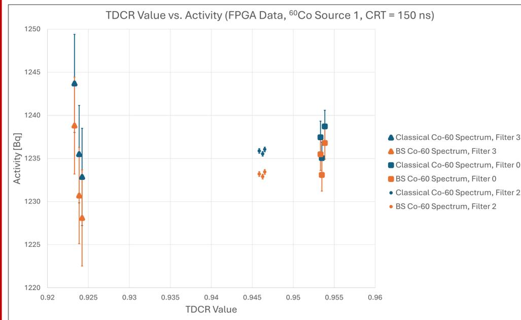
Figure 2: Calculated activity [Bq] as a function of the measured TDCR value calculated using FPGA acquired data for  $^{60}\text{Co}$  Source 1 and a CRT of 150 ns with different filters applied
