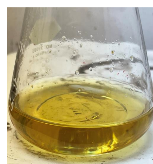
*Figure 3: Example of cellulose completely dissolved in 25% NaOH
