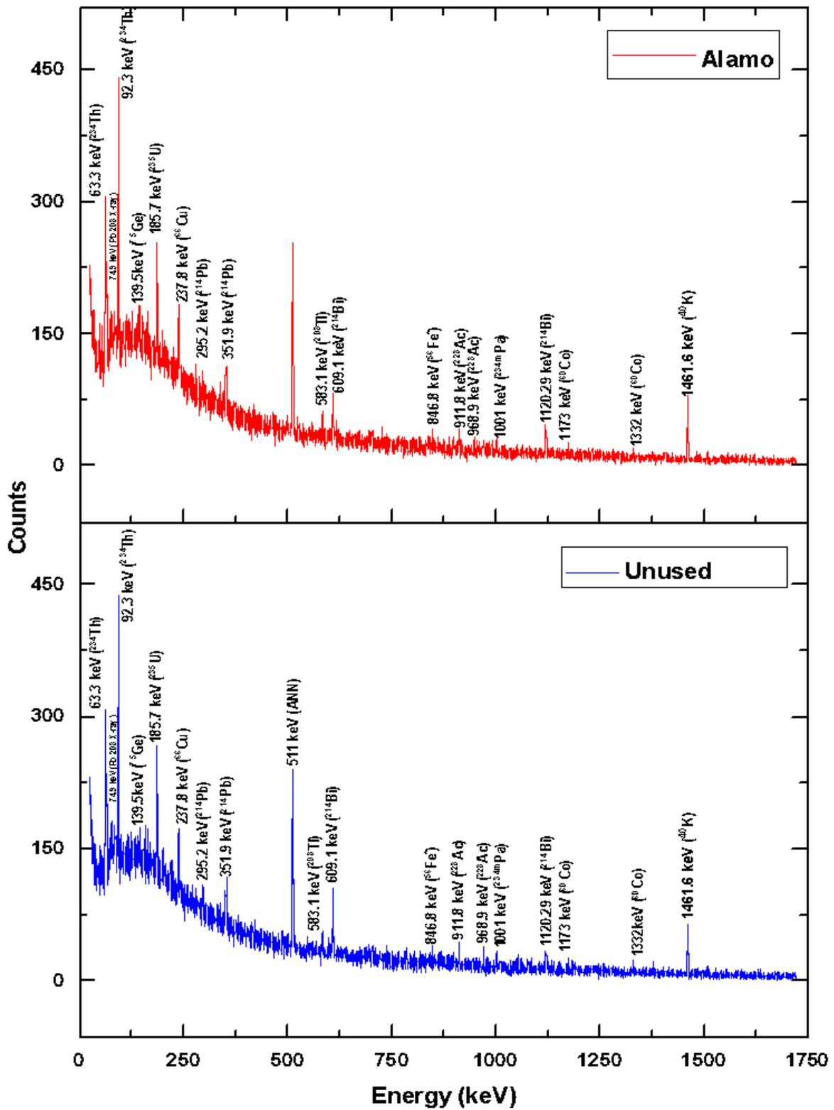
Figure 3. Comparison of Gamma spectra of typical unused filter paper and the filter from the Alamo CEMP station
