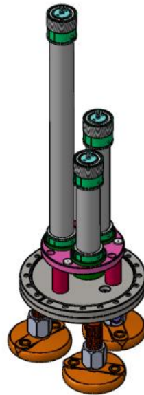
Figure 1: CAD drawing of length-compensated proportional gas counters at NIST. This system will be placed in a manifold and exposed to a combination of source and counting gases.
