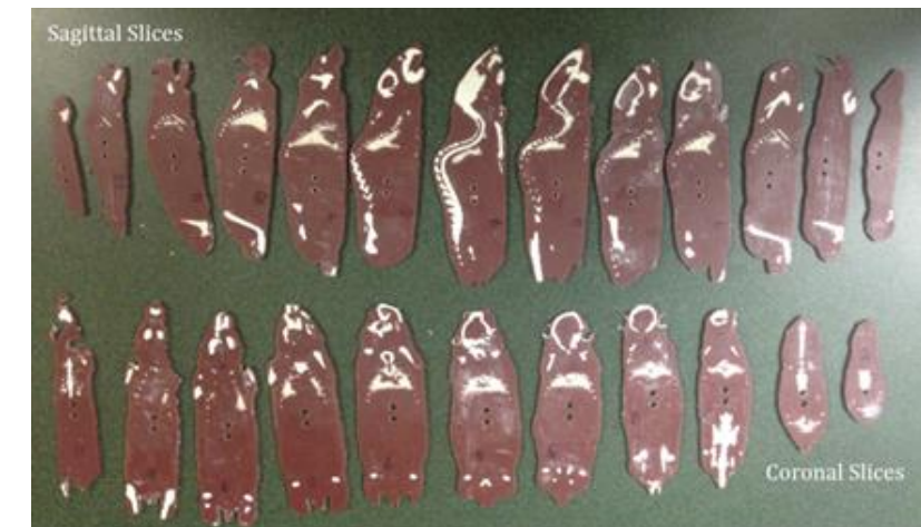
Univ of Wisc. phantom with real rat skeleton and TLD cavities
