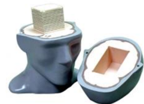
Univ of Wisc. phantom with real rat skeleton and TLD cavities
