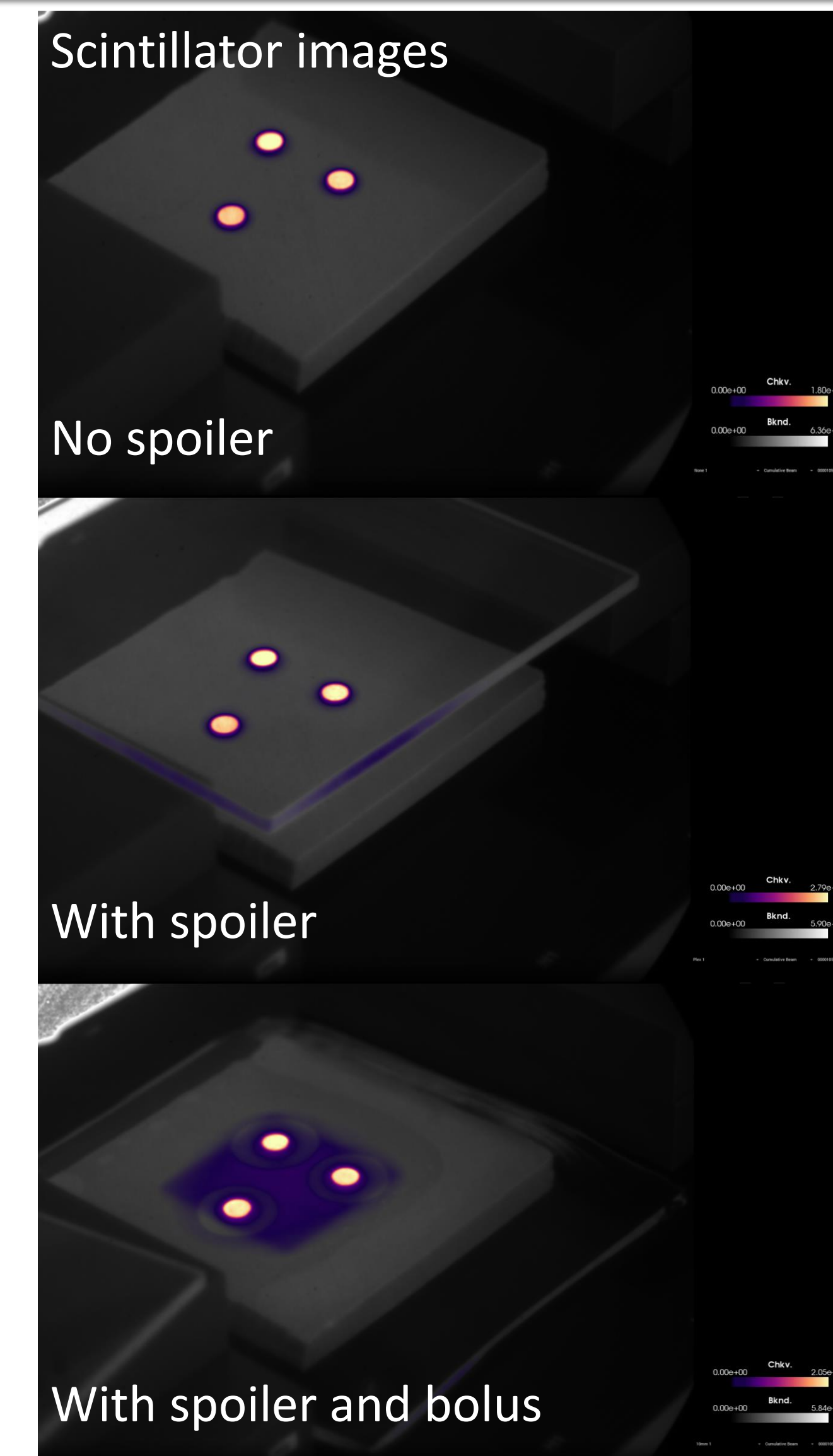
Figure 5: C-Dose images of scintillators on a flat plane without the plexiglass spoiler, with the spoiler, and with the spoiler and bolus
