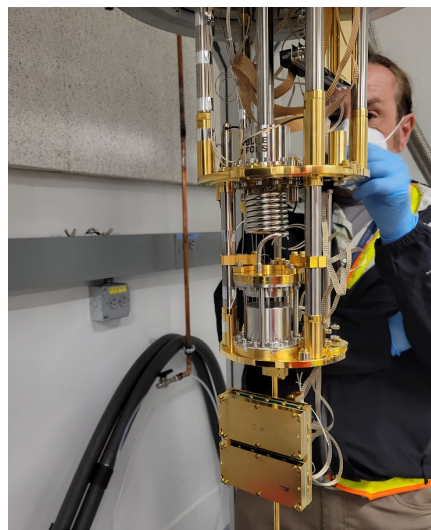
Dan Schmidt and Ryan Fitzgerald installing TES sensors and first quantitative alpha sources
