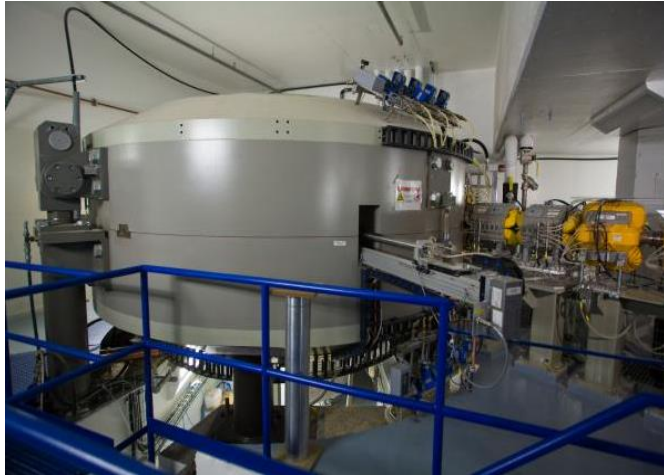
Laser plasma accelerator, <25 MeV, 10^9 Gy/s in pulse
