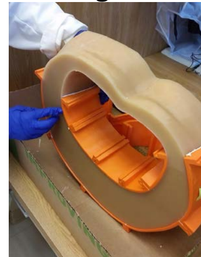
Demolding after overnight cure
