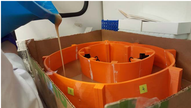
Casting using polyurethane rubber
