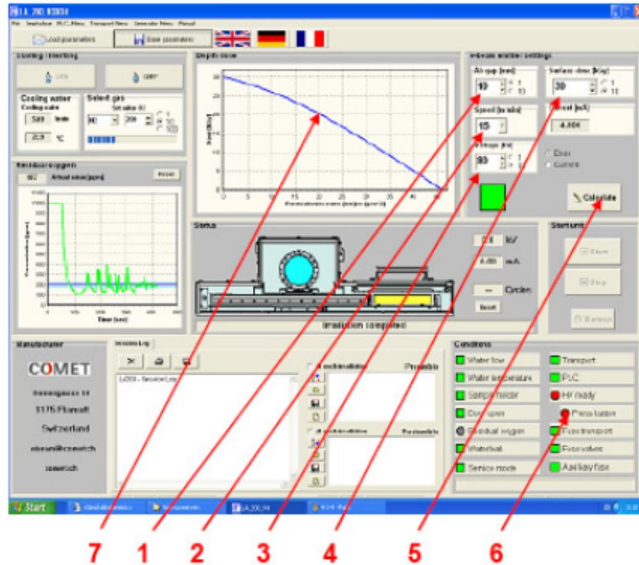
1. Air gap between ebeam lamp window and sample material (where dose is deposited)
