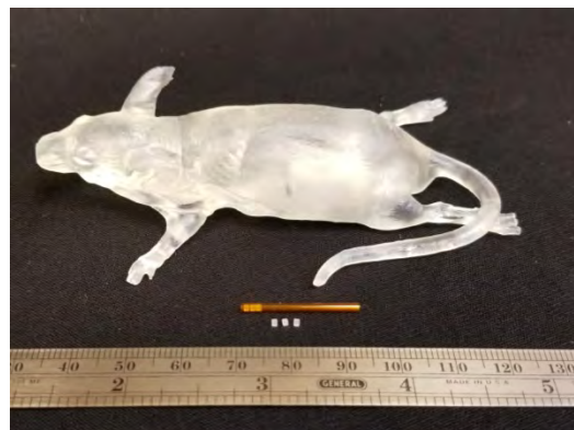
Figure 1: A 3D-printed murinemorphic phantom was fabricated. They were printed using Formlabs clear resin with a void for kapton tubes loaded with TLD-100 microcubes.
