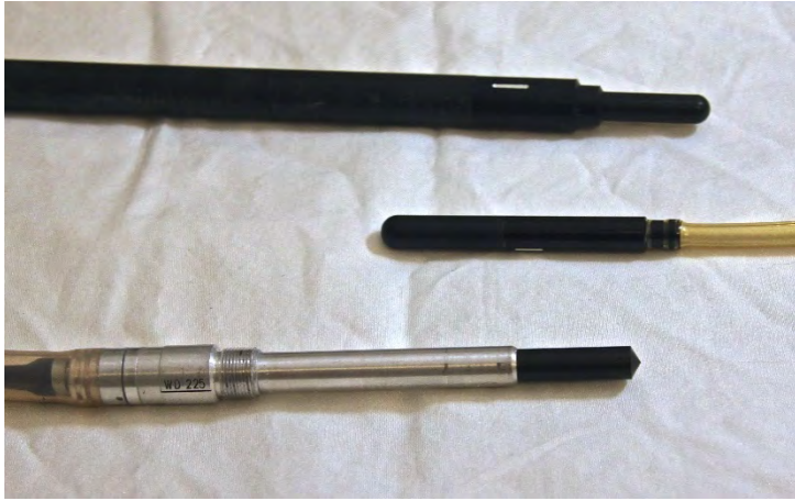
Figure 1: Exradin A12 Farmer chamber (top), Exradin A28 scanning chamber (middle) and Wellhofer IC69 Farmer chamber (bottom) that were calibrated at the NRC.
