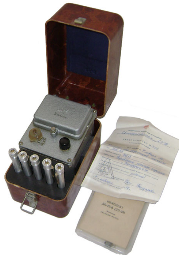
Set of 5 Soviet personal radiation dosimeters DP-24 Image from: http://www.soviet-power.com/detail.php?pid=45138
