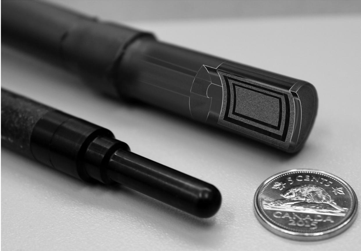
FIG. 1. The comparable size of the Aerrow to that of a Farmer-type ionization chamber is illustrated by the Exradin A12 positioned alongside the probe calorimeter (internal Aerrow structure is shown as a blended rendering) and a 5-cent coin (21 mm wide) for scale.
