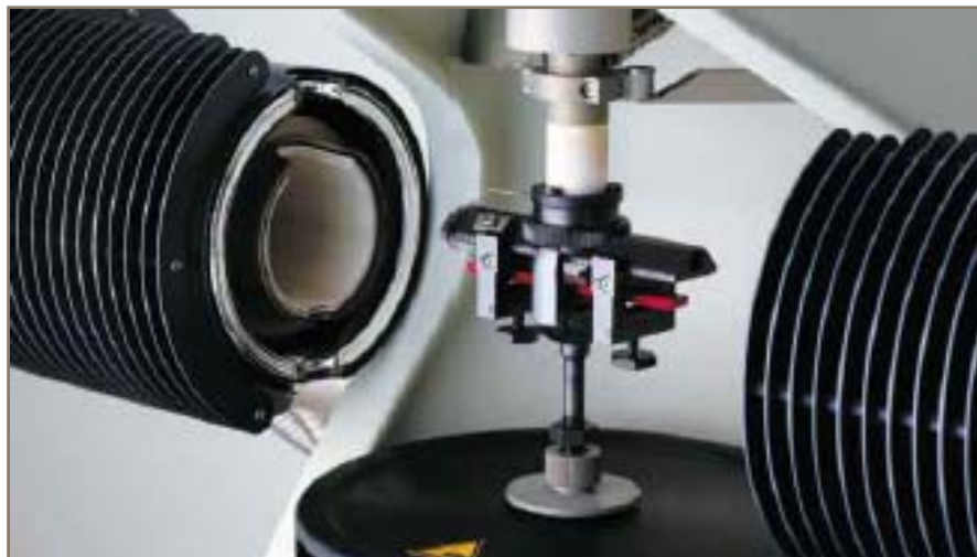
DMA 3 point bend fixture – Load Cell: 40N, multi-frequency
