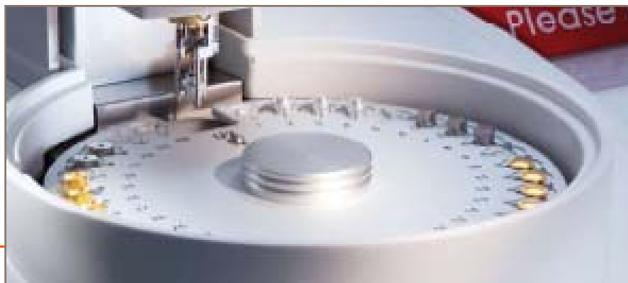
DSC Robotic Autosampler – Temp range -100 °C to 700 °C
