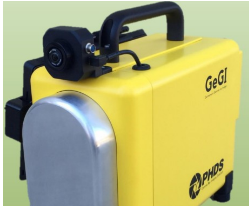
GeGi: segmented HPGe detector
