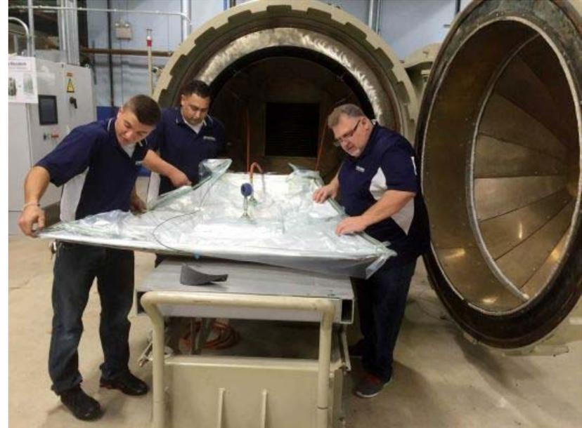
**Composite Prototyping Center 2.4 m diameter, 6.1 m long autoclave**
