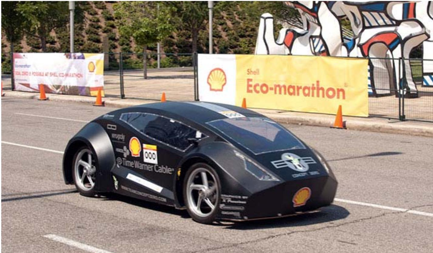
**Concept Zero – 103 kg carbon fiber prototype vehicle
