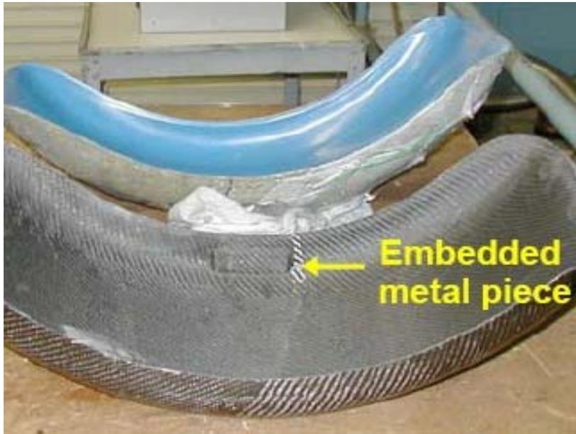
**Cured fender with metal piece embedded between plies**
