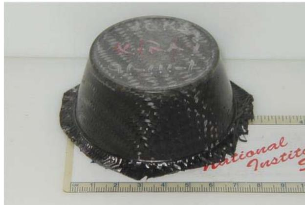
**Carbon fiber shape X-ray cured in the mold**
