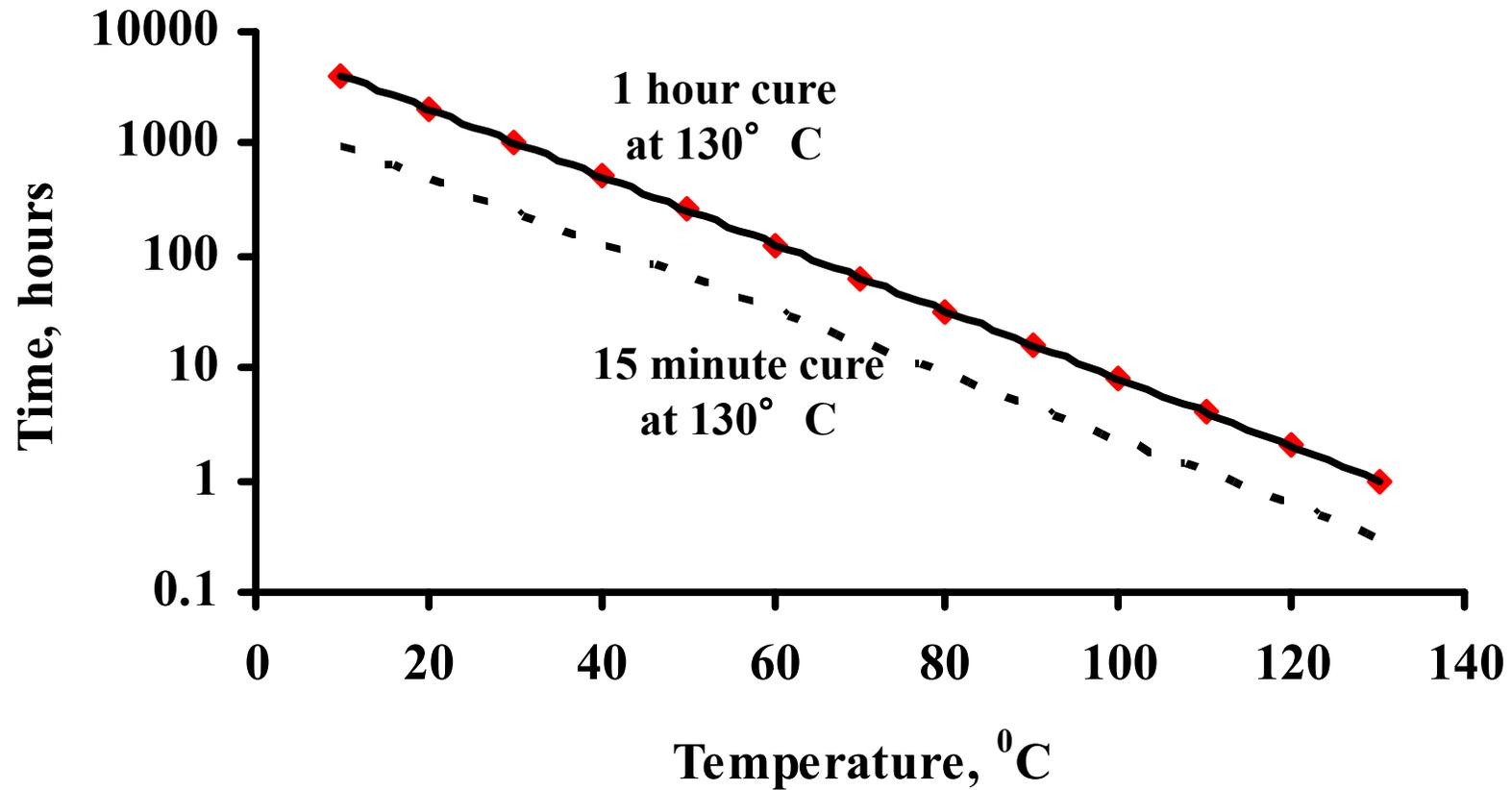
Thermoset curing reaction kinetics – time at temperature
