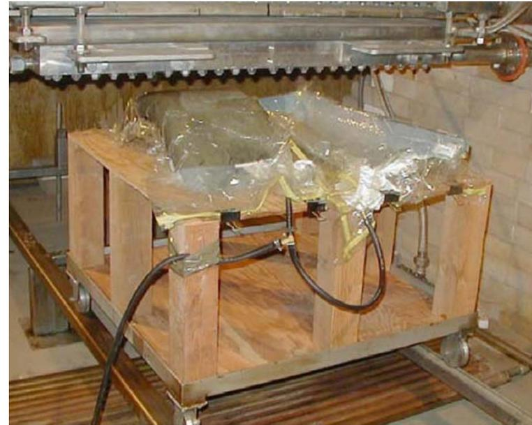
**X-ray curing motorcycle fenders in molds**
