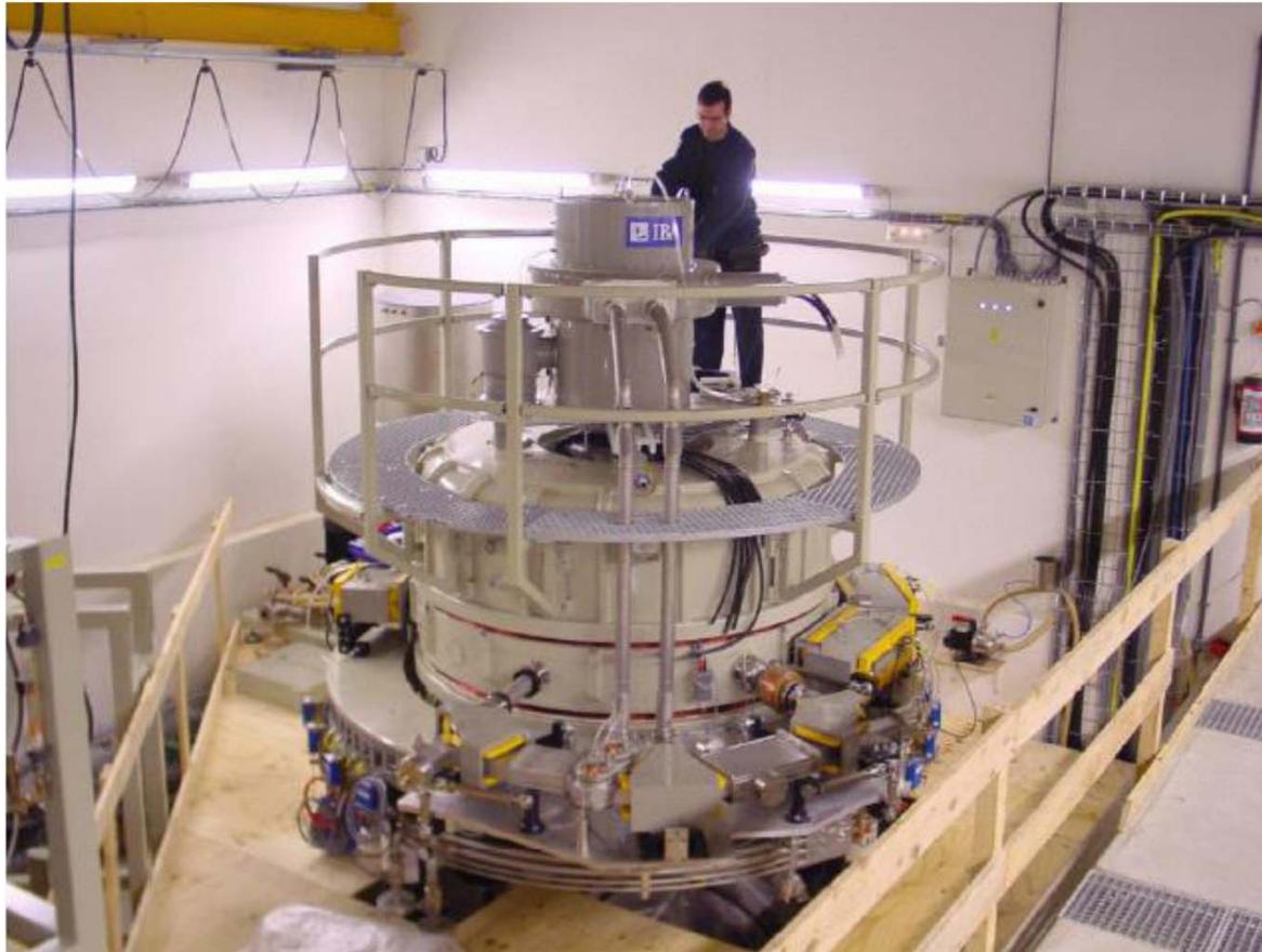
**7 MV 700 kW EB accelerator X-ray treatment in use since 2010**
