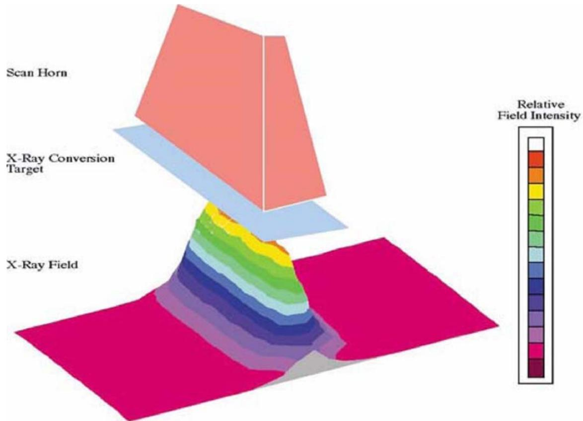
**Water cooled Tantalum target interposed between
