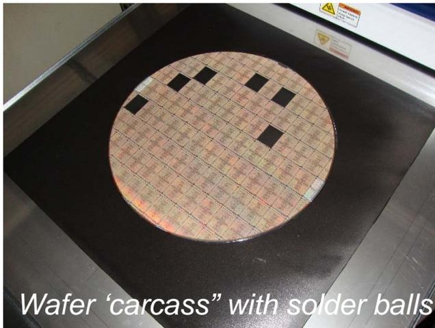
*Wafer 'carcass' with solder balls*
