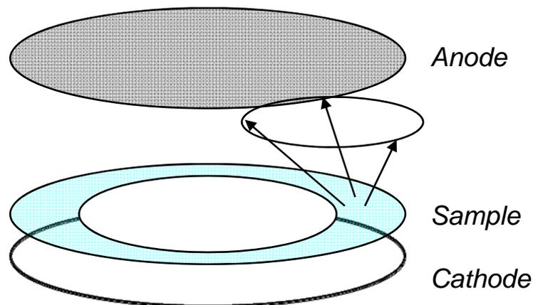
*Vector represents  $\alpha$ -particle track length in counter gas (function of gas pressure and alpha particle energy)*
