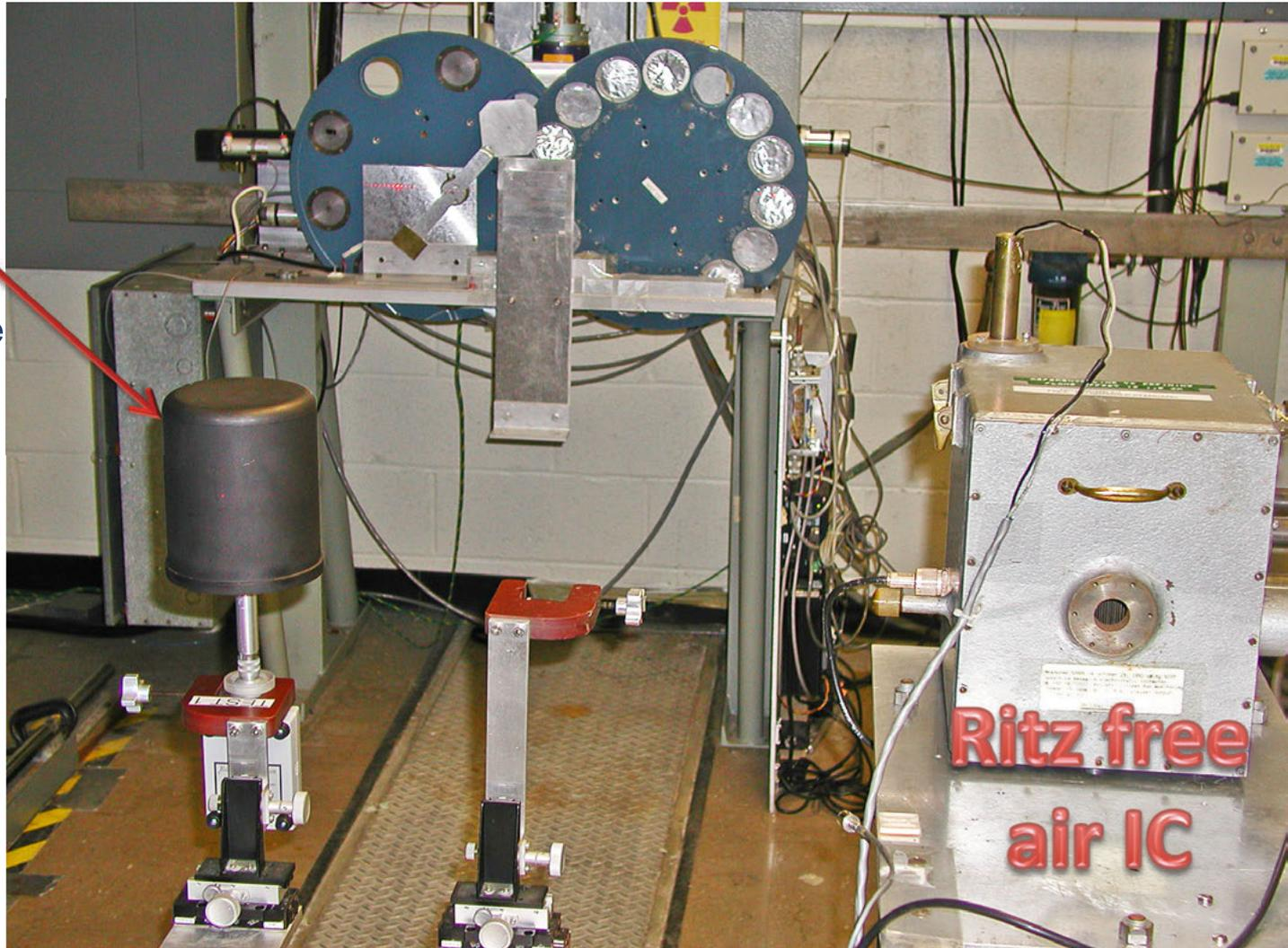
...performed by chamber substitution, with standard beam qualities
