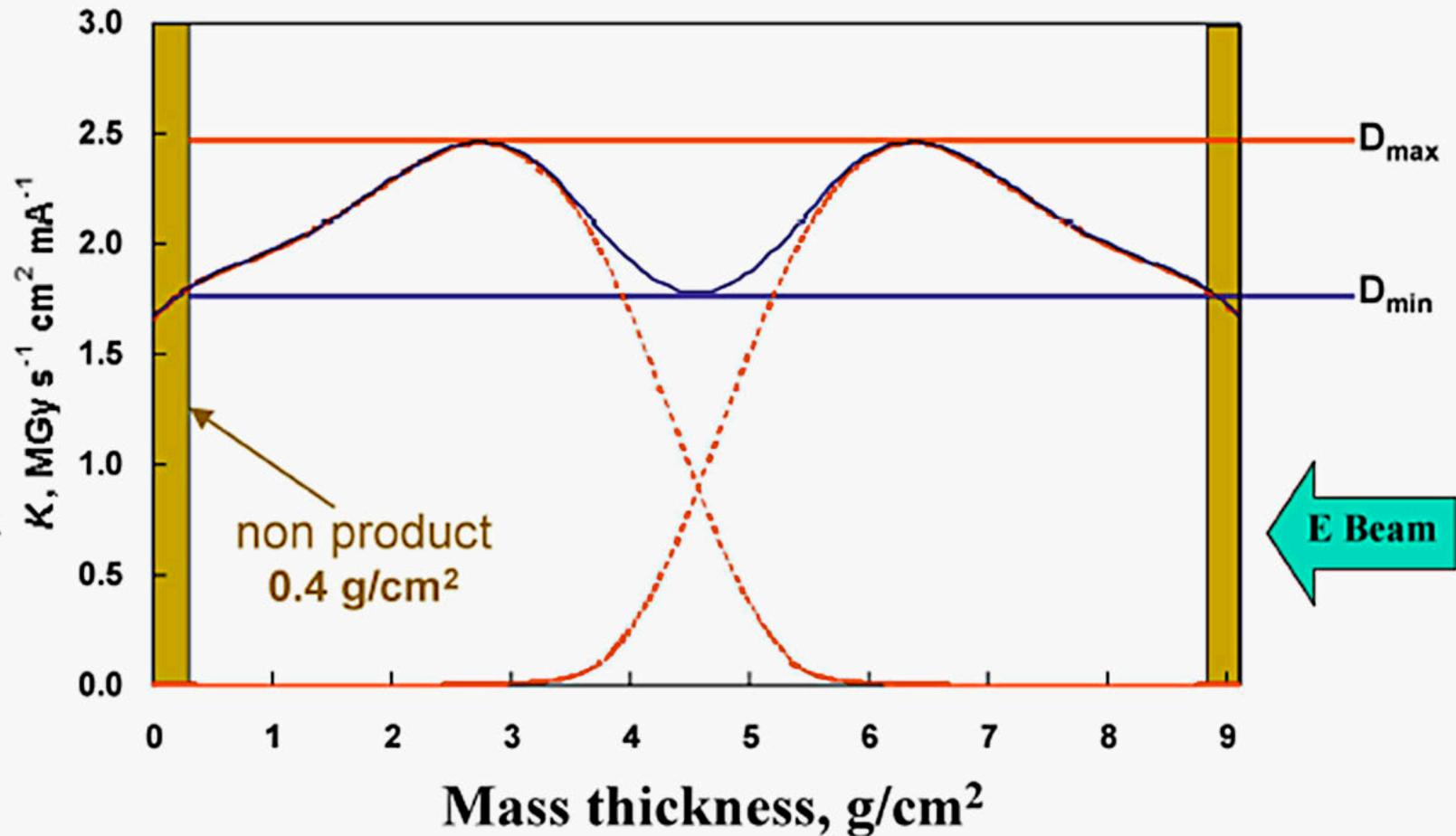
Task: tune product depth and irradiation parameters to achieve the most efficient & uniform dose distribution
