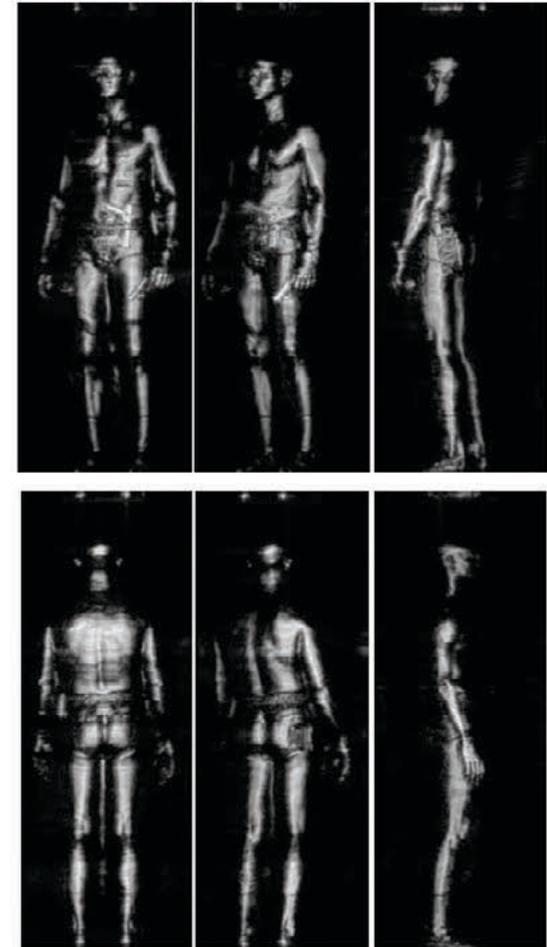
Figure 4 Wideband (27 - 33 GHz) images of a man carrying two concealed handguns along with several innocuous items.
