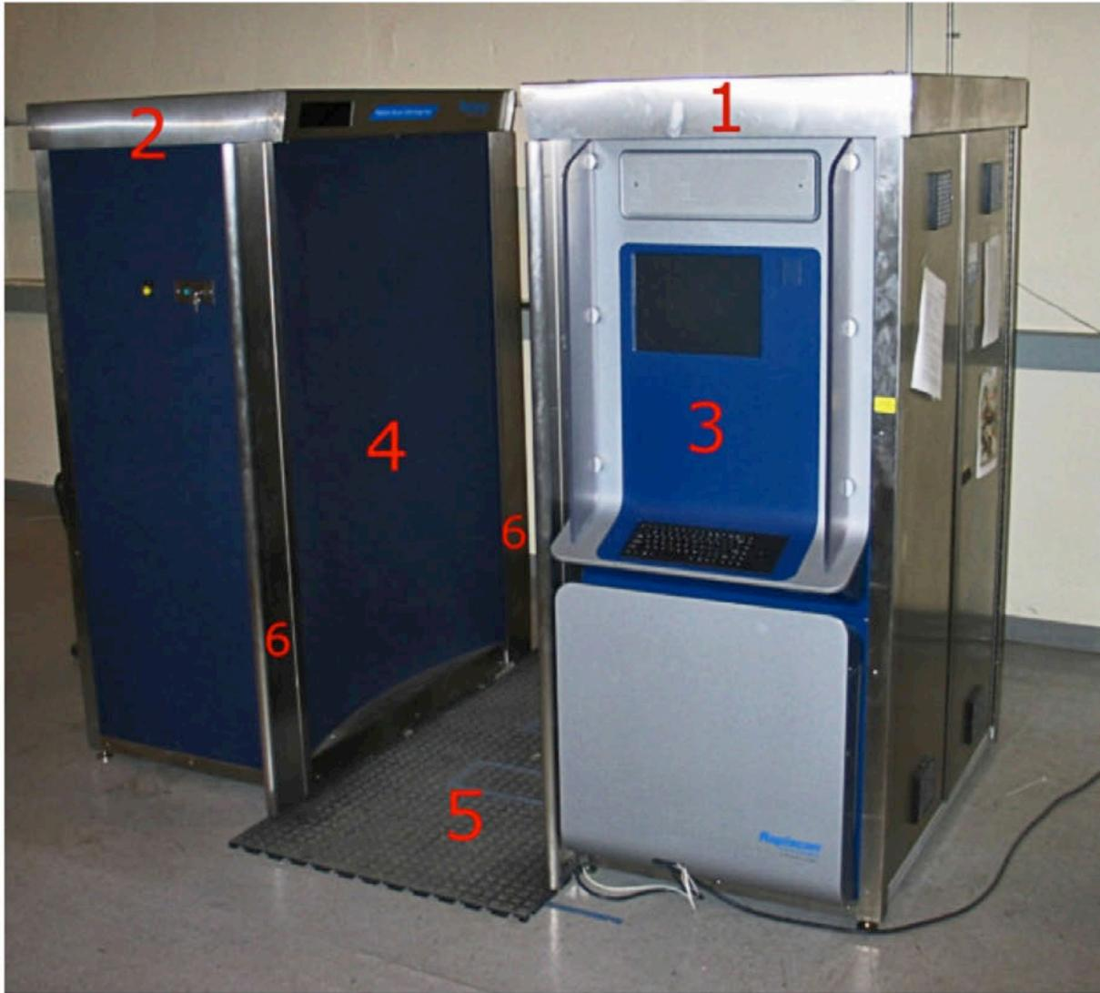
(1) master scanner; (2) slave scanner; (3) operator console; (4) front panel of the slave scanner; (5) floor mat; (6) wings of the slave scanner.
