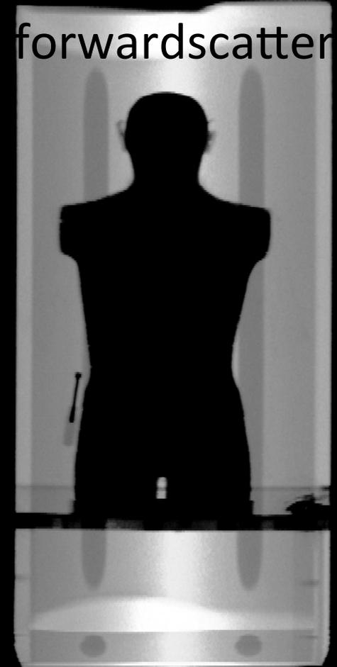
For a constant x-ray energy, low-Z materials (*e.g.* organics) Compton scattering dominates so brighter in backscatter; for higher-Z materials (*e.g.* metals) the photoelectric effect dominates, so darker in image.
