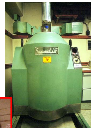
Co-60 Irradiator, NIST ( \gamma irradiator)
