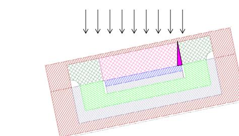
The Guard's Volume is attenuating a portion of the Collector's Volume (in 3D, it doesn't take much to lose a measurable portion of the signal).
