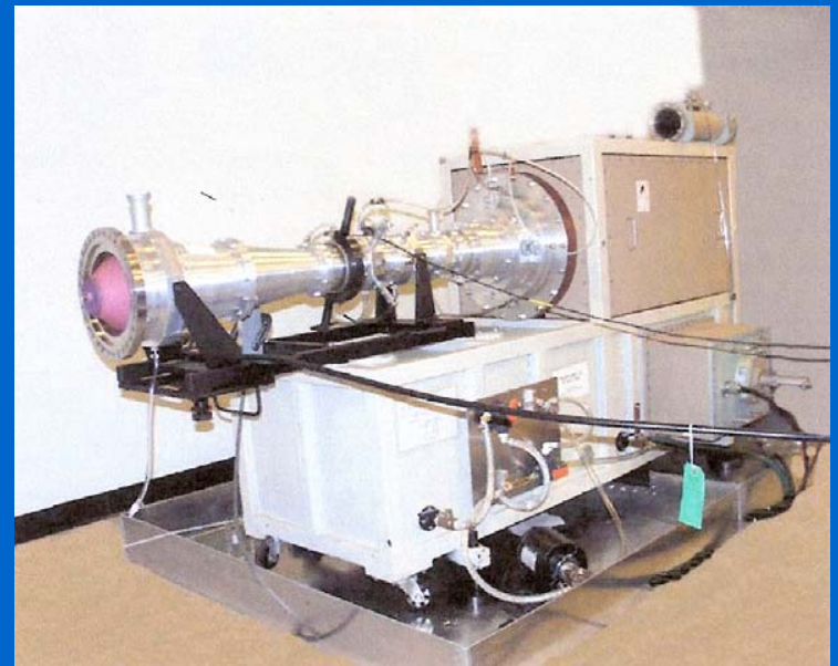
5 MV Pulsed Power Supply System
