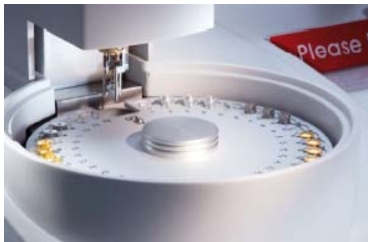
DSC Robotic Autosampler – Temp range -100 °C to 700 °C
