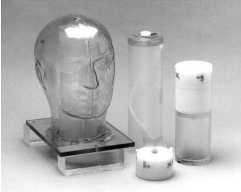
Image of phantom (left) evaluated with imaging insert (center) and dosimetric insert (right)
