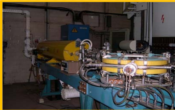
7.5 Mev Dual Energy Accelerator - 2005
