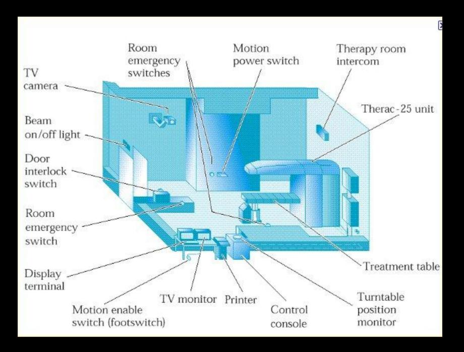
On July 26, 1985; a patient received an over exposure at the Ontario Cancer Foundation in Ontario, Canada. A defect in the computer program controlling the Therac-25 radiation therapy accelerator resulted in an overexposure to a patient. A 40-year old woman being treated for cancer received a localized dose
