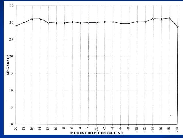
Electron beam scan pattern obtained using a strip of polyethylene dosimeter material
