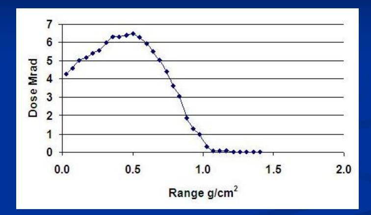
Depth-dose curve obtained using a polyethylene depth-dose pack
