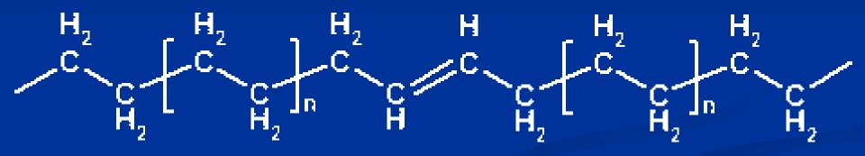
Transvinylene double bond in irradiated polyethylene
