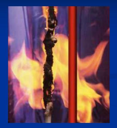
Flammability test: flame retarded irradiation crosslinked wire jacketing does not drip or fall away from the conductor
