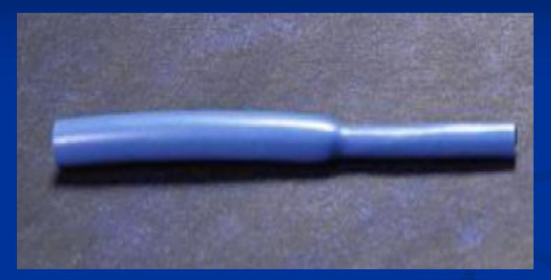
Too high a hot modulus = difficulty expanding the tubing = possible spitting on recovery Too low a hot modulus = insufficient recovery force
