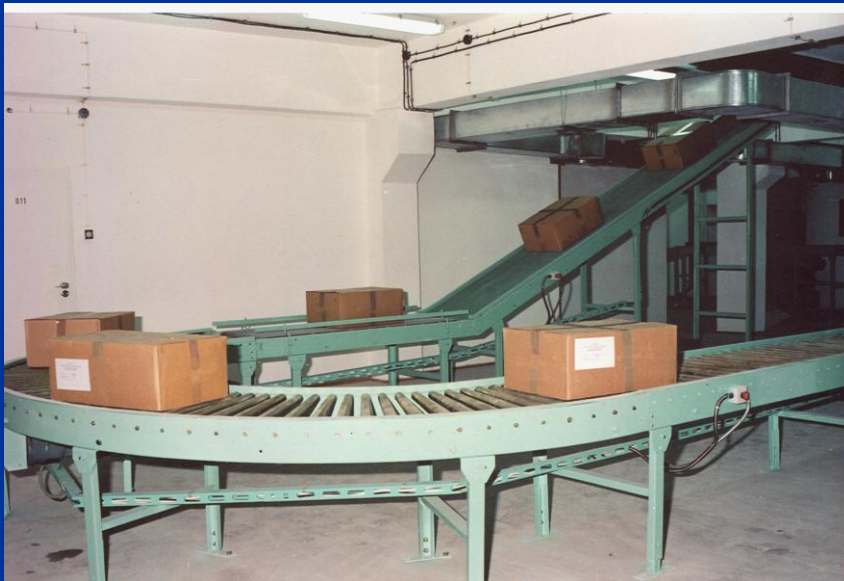
Conveyor system with prepacked spices in boxes
