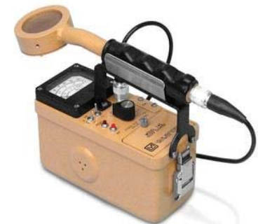
Ludlum model 14-C with pancake probe
