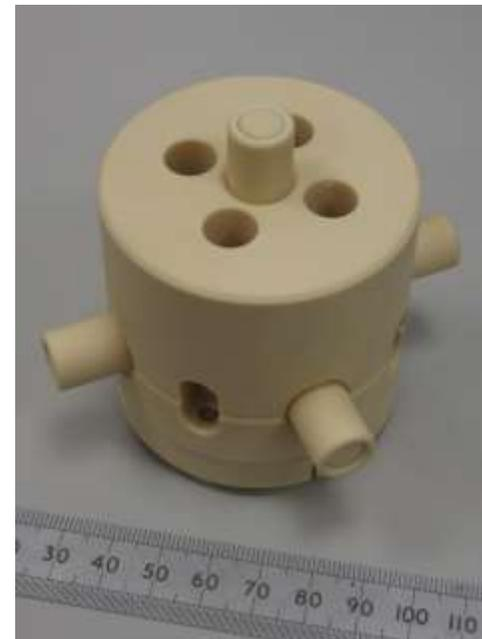
**Intrabeam phantom 2** with alanine pellets at 5, 10 and 15 mm distance from surface of 40 mm spherical applicator
