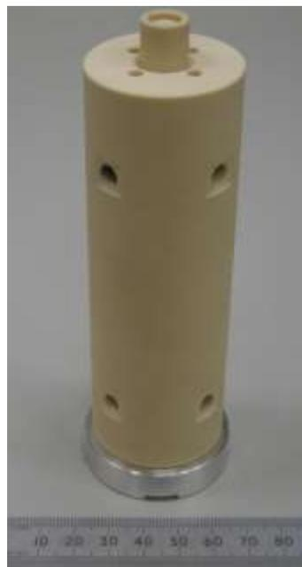
**Intrabeam phantom 1** with alanine pellets at 5, 10, 20, 30 and 40 mm distance from end of bare needle
