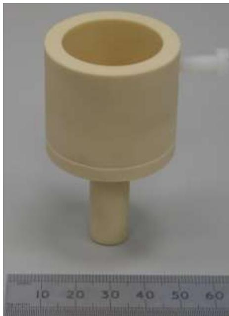
**Papillon 50 phantom** with alanine pellets at 0, 5, 10, 15, 20 and 25 mm distance from end of 25 mm diameter applicator tube
