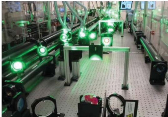
Laser plasma accelerator, <25 MeV, 10^9 Gy/s in pulse
