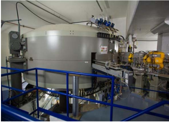
Laser plasma accelerator, <25 MeV, 10^9 Gy/s in pulse
