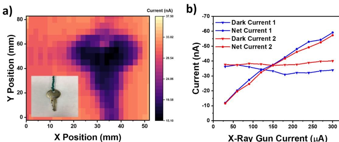
Figure 2. a) X-ray image of a brass key from MAPB, b) Repeated current vs. X-ray flux measurements showing relatively stable sensitivity
