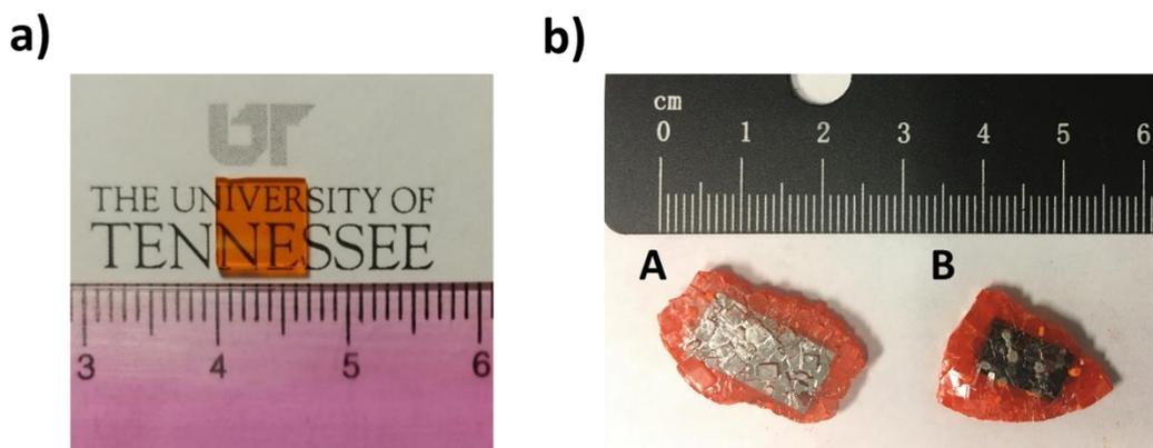
Figure 1. a) MAPB single crystal, b) Fabricated polycrystalline MAPB detectors
