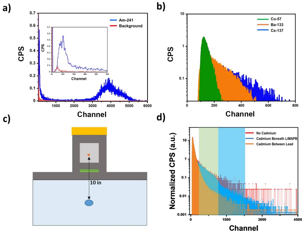
Figure 3. a) Alpha peak and X-ray photopeak (insert) from a non-spectroscopic  $^{241}\text{Am}$  smoke detector source observed in  $\text{MAPbBr}_{2.85}\text{Cl}_{0.15}$ , b) Background subtracted spectra from various gamma ray sources with LiMAPB, c) Shielding arrangement for LiMAPB thermal neutron sensing with PuBe (dark blue), HDPE (light blue), lead (gray), cadmium (green), and paraffin (yellow), d) LiMAPB response to PuBe with multiple shielding configurations
