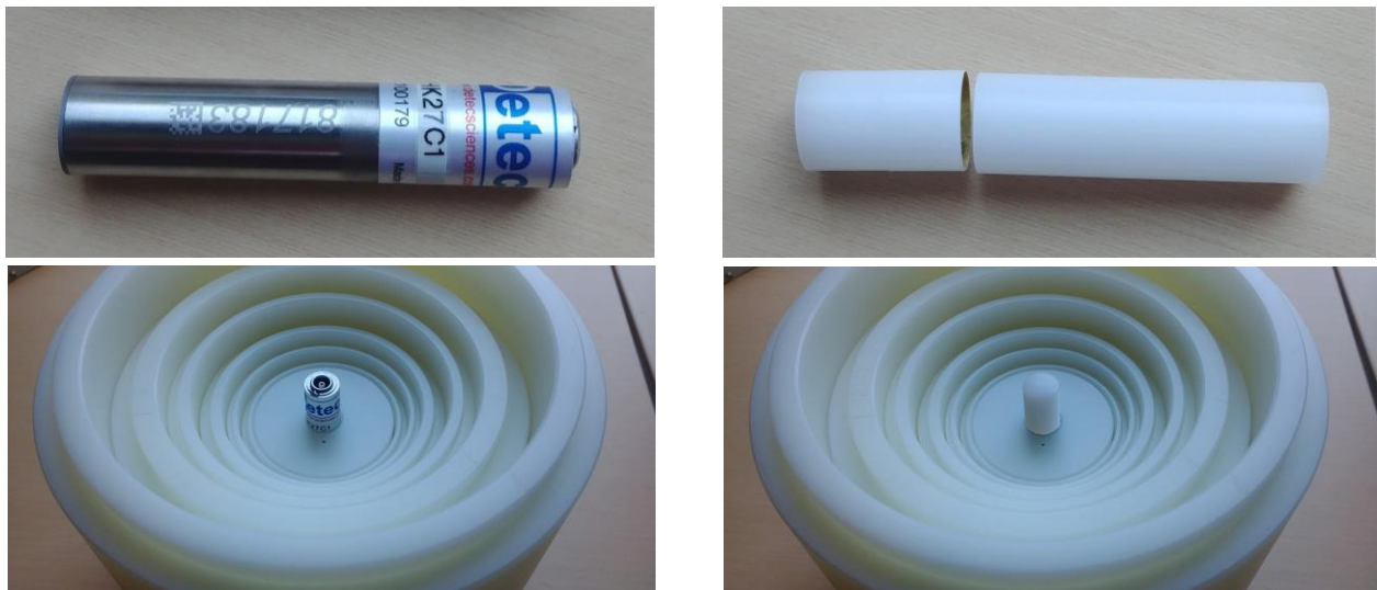
Figure 1. The He-3 detector and its positioning inside the nested moderators of the NNS (left). The picture of the two cylindrical insert with the gold foil inbetween and its positioning inside the moderators to have a passive NNS (right).
