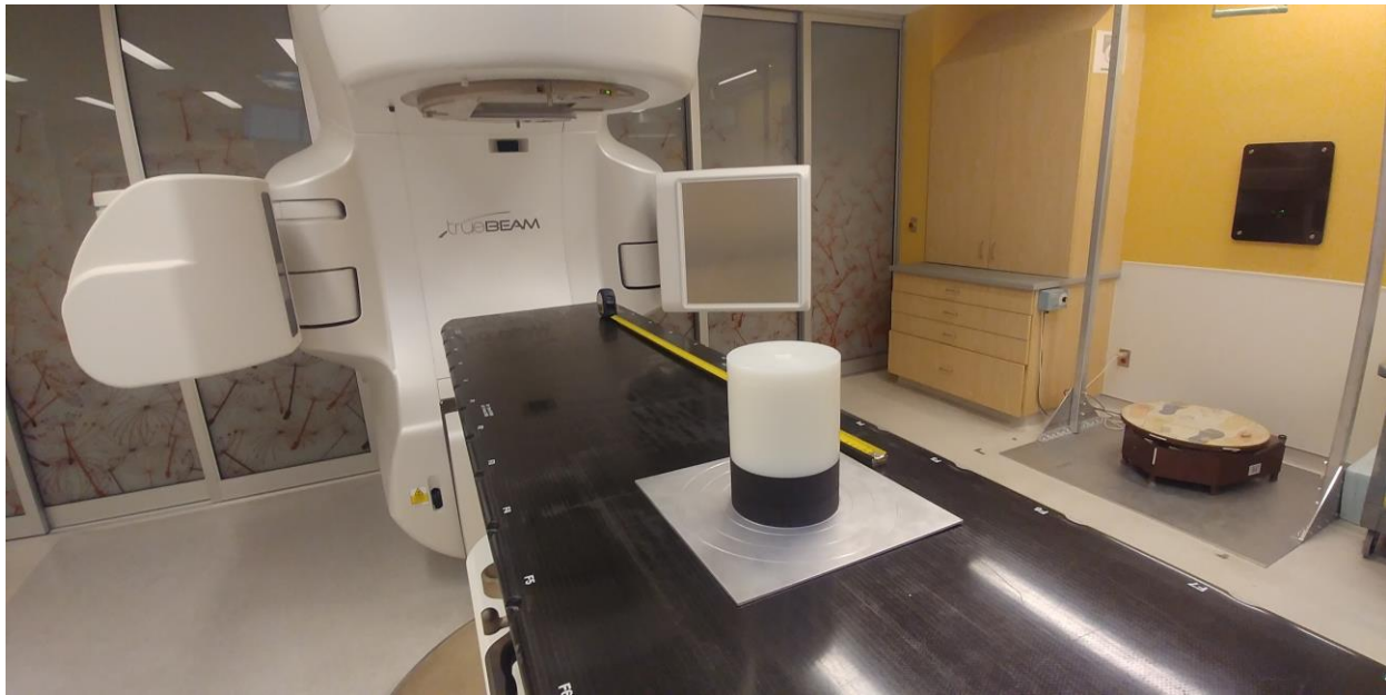
Figure 2. The passive NNS with gold foil in one of its moderator configurations at the location of measurement in the radiotherapy bunker during irradiation.
