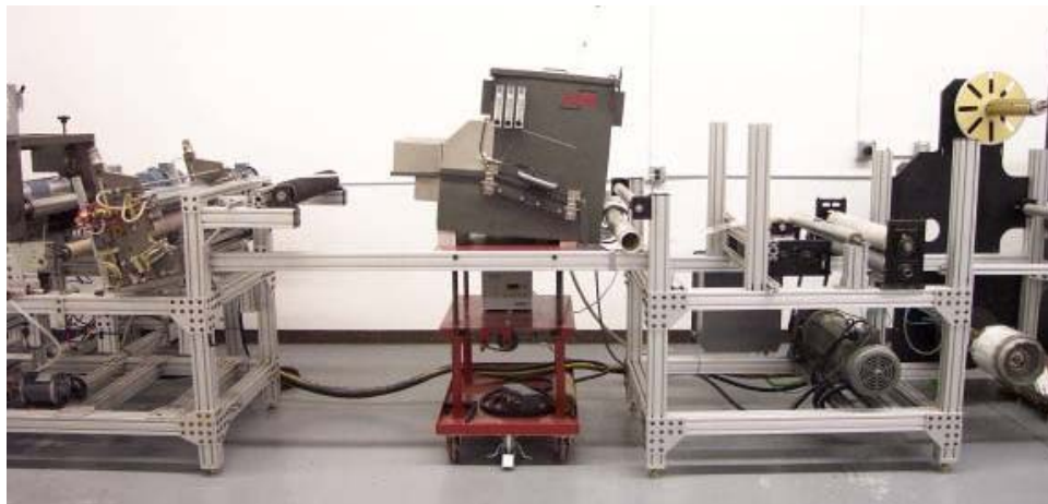
Figure D.8.0b - Low-voltage electron beam on coating pilot line (courtesy of Advanced Electron Beams, Incorporated)
