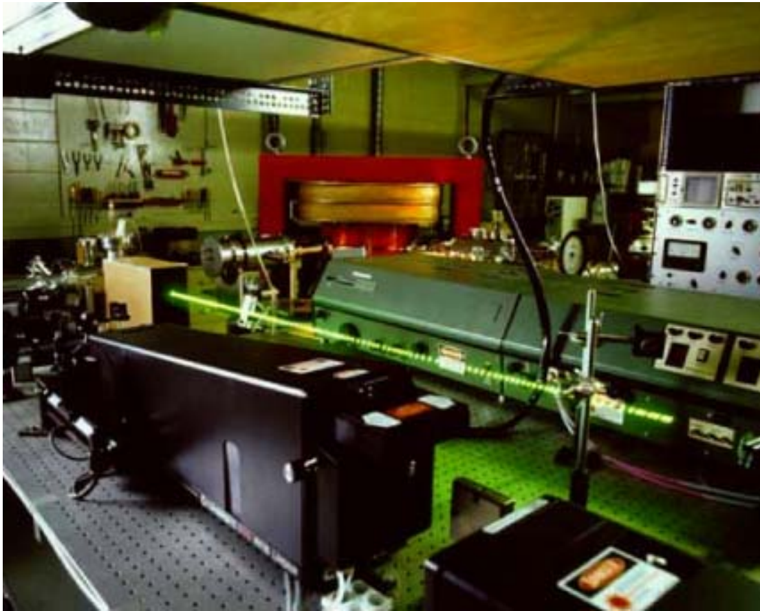
Figure B.9.1 - Resonance ionization mass spectrometry (RIMS) system (courtesy of NIST Ionizing Radiation Division)
