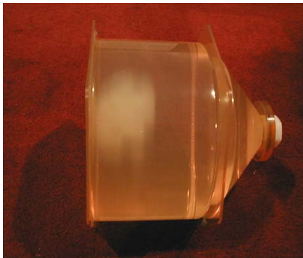
Figure A.3.3a - Irradiated BANG gel dosimeter (courtesy of MGS Research, Incorporated)
