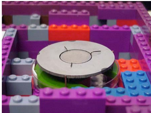
Figure D.8.0a - Low-voltage electron beam calorimeter (courtesy of Risø National Laboratory, Denmark)
