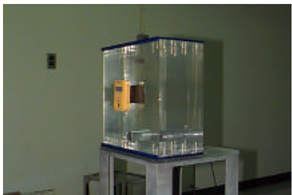
C.18.1 Electronic personnel dosimeter on a lucite slab for calibration in a beam at Battelle Pacific Northwest National Laboratory.
