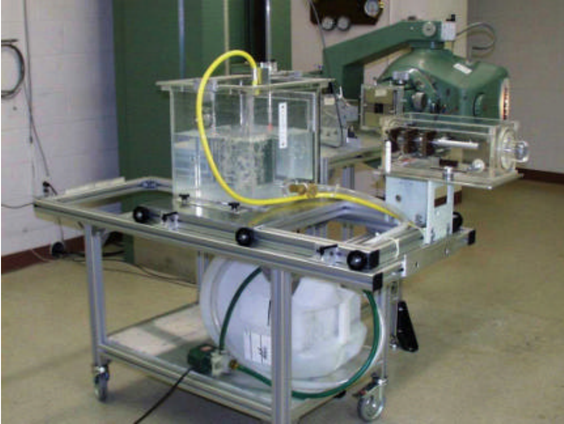
A.4.1 Water phantom set up for absorbed dose to water measurements at the K&S Accredited Dosimetry Calibration Laboratory.
