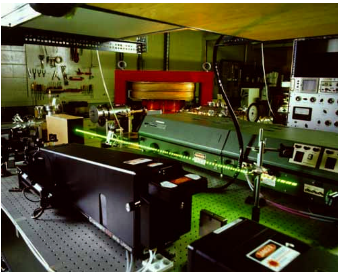
B.4 Resonance ionization mass spectrometry (RIMS) system at the National Institute of Standards and Technology.
