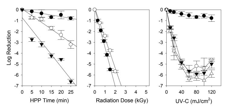
Inactivation of Uropathogenic E.coli on chicken meat and chicken purge by nonthermal processing technologies. HPP 300 ( $\bullet$ ), 400 ( $\circ$ ) and 500 ( $\blacktriangledown$ ) MPa are shown as well as gamma radiation at 4 ( $\bullet$ ) and -20 ( $\circ$ ) oC. For UV-C inactivation of UPEC on chicken breast meat ( $\bullet$ ), and chicken exudates on SS ( $\circ$ ), HDPE ( $\blacktriangledown$ ) and HDPP (). Each experiment was conducted independently three times (n=3).
