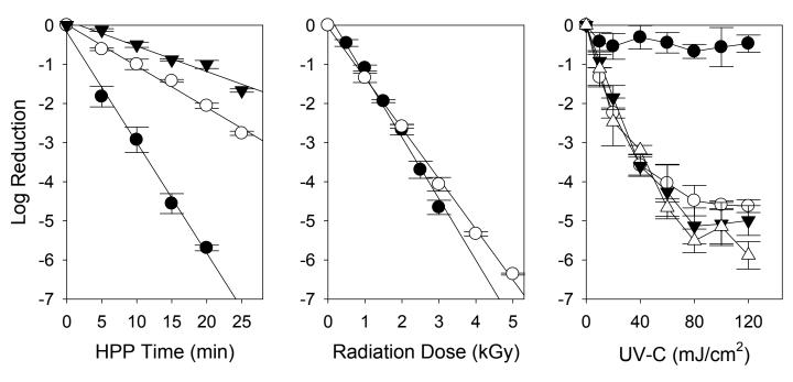
Inactivation of S. saprophyticus on chicken meat and chicken purge by nonthermal processing technologies. HPP 300 ( $\bullet$ ), 400 ( $\circ$ ) and 500 ( $\blacktriangledown$ ) MPa are shown as well as gamma radiation at 4 ( $\bullet$ ) and -20 ( $\circ$ ) oC. For UV-C inactivation of UPEC on chicken breast meat ( $\bullet$ ), and chicken exudates on SS ( $\circ$ ), HDPE ( $\blacktriangledown$ ) and HDPP (). Each experiment was conducted independently three times (n=3).
