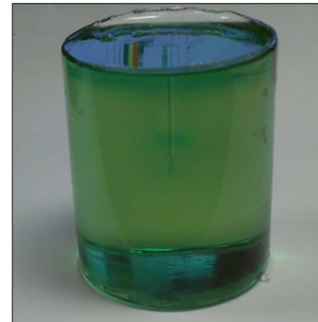
Figure 2. Presage® dosimeter with channel in center for I-125 seed placement
