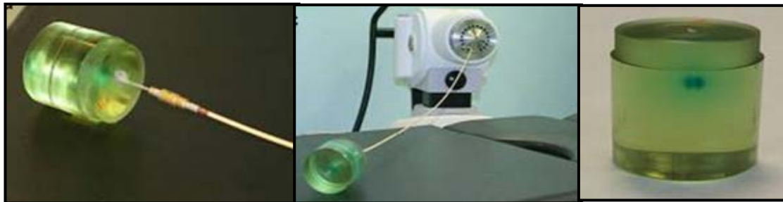
Figure 1. PRESAGE® dosimeter connected to remote afterloading device to expose Ir-192 source at end of catheter
